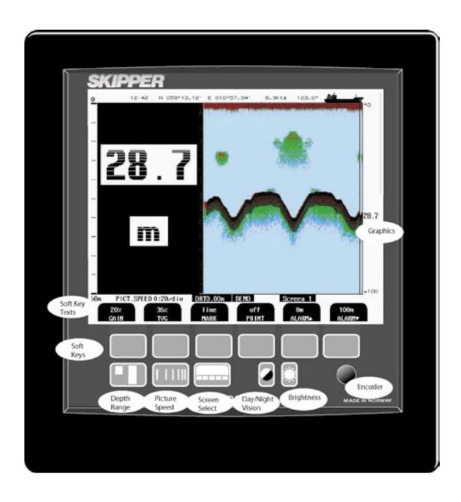
Fig. 1.1 Main Display Unit Panel Layout
