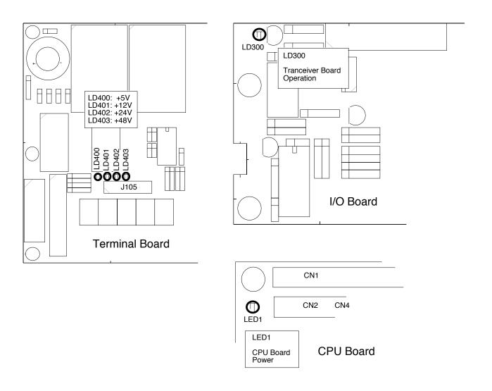
Fig. 4.6 Function LEDs, Terminal, I/O and CPU Boards.
