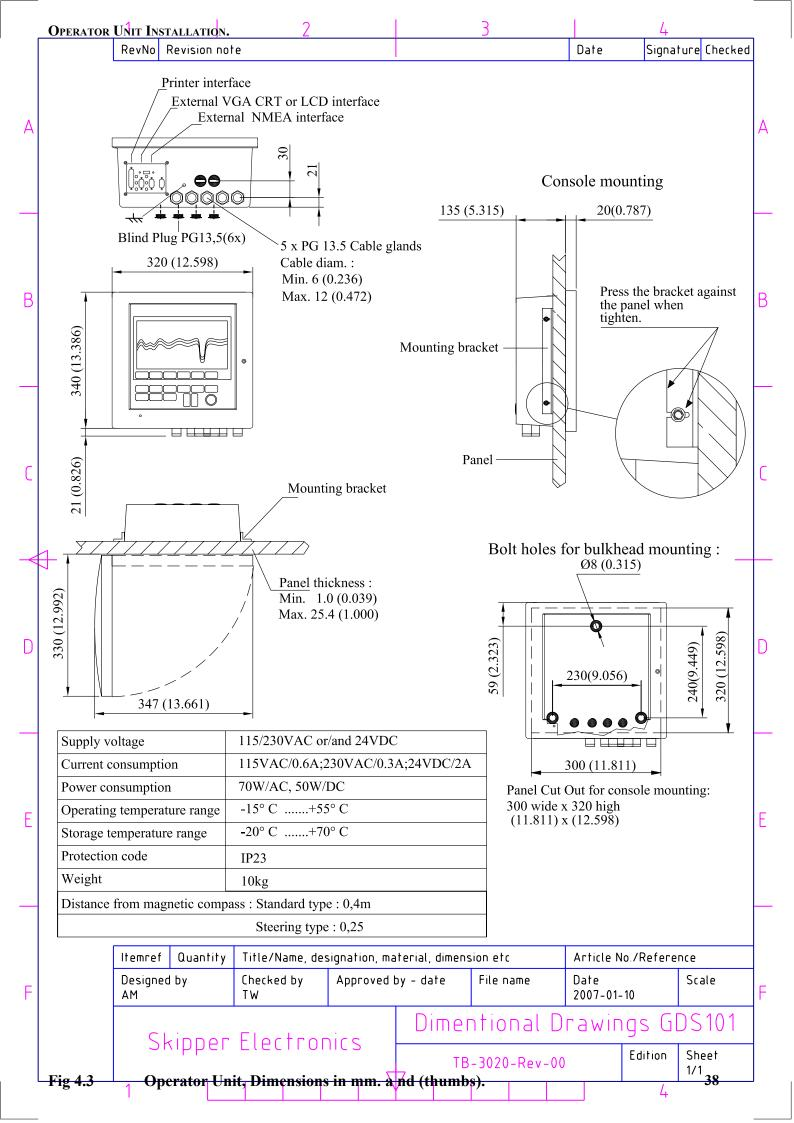
Select a position to provide free view of the panel as well as easy access during operation and service. The operator unit may be mounted flush in a panel or directly onto a bulkhead. Fig.4.3 shows the operator unit along with the main installation dimensions.
