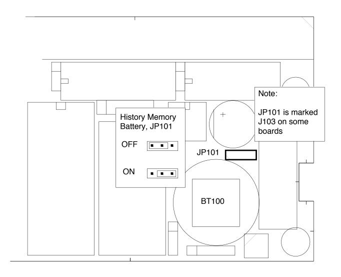
Fig. 4.5 History Memory Battery Jumper, I/O Board.
