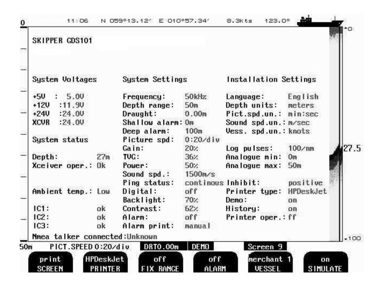
The status Screen (9) contain information that will faciliate analysis and correction of several problems. A printout of the Status and Oscilloscope Screens should be sent by fax with any report about functional Disturbance. This will greatly facilitate remote failure Analysis.
