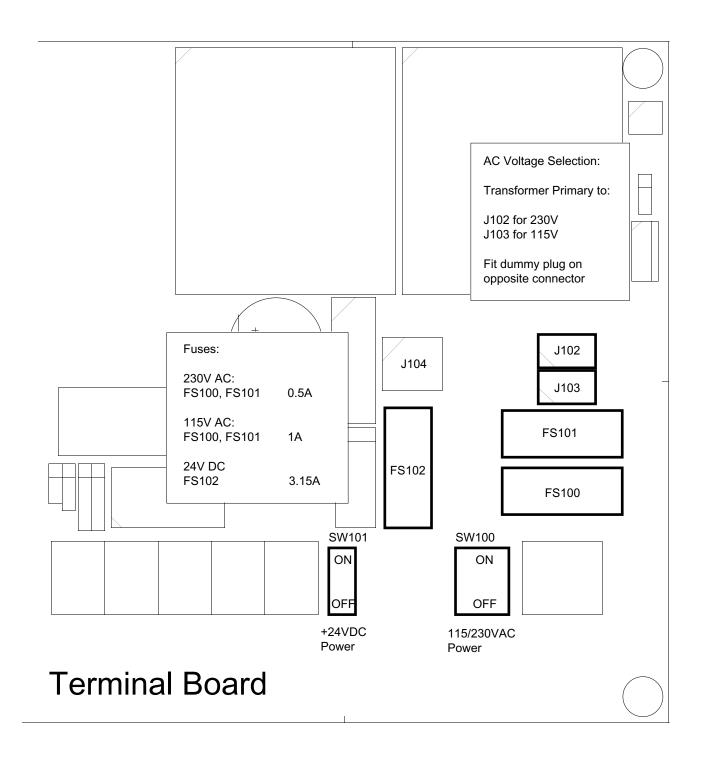
Fig. 4.4 Voltage selection connectors and fuses, Terminal Board.
