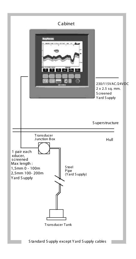
Fig. 4.1 Basic System Configuration.
