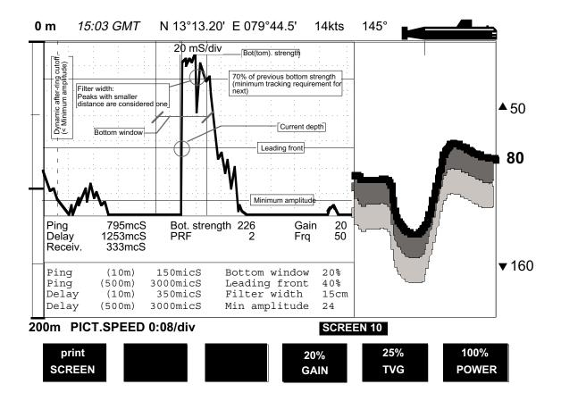
This Oscilloscope Screen (10) shows a typical oscillogram of a bottom echo (the tall peak in the centre of the diagram) and a weaker fish echo to the left of it. The horizontal axis represent time for the sound to travel down and back from an object. The vessel is located at the left edge of the grid, and the right edge represent the deep range. The vertical axis represent the magnitude of the echo signal received.
