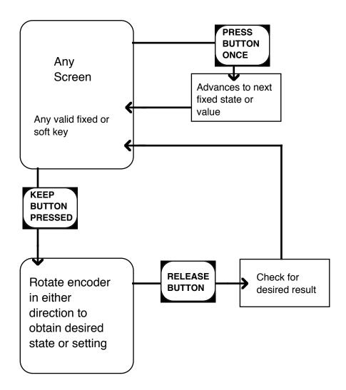
Fig. 2.1 Setting and Parameter Entry Flowchart
